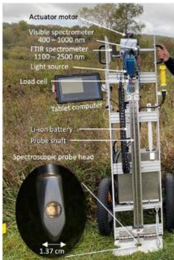
Figure 3.2.1. Subterra Green prototype (TRL 5-6) from S4ML
